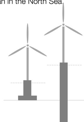
Picture 2. Gravity foundation left, monopile right.
